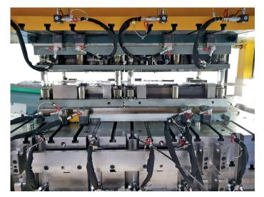
Sliding clamp with T-slot adapter in press bed and ram
