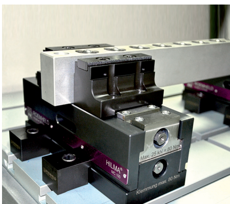
Clamping of aluminium bars with workholding system MC-P 100 Z Balance.
