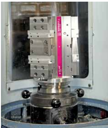
Tower workholding system TS 80 TriStar, a workholding system with connection to Matsurra MAM 72
