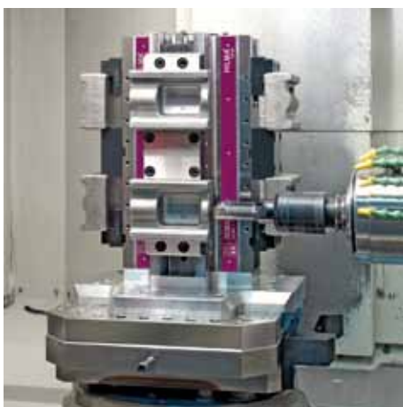
Tower workholding system TS 125 with 3rd-hand function
