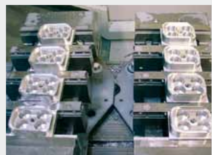
The clamping step edge is milled off in the 2nd clamping step.
