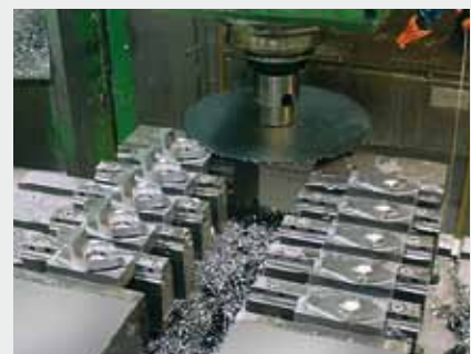
After finish-machining, the "lost head" is separated from the workpiece using a disk milling cutter.
